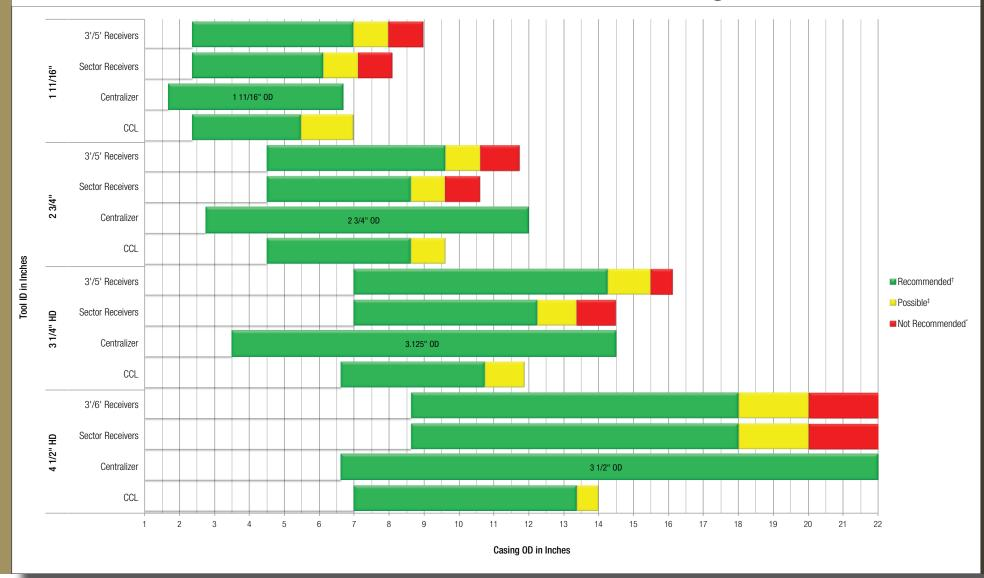
Due to variables such as well bore fluid density, casing weights and tool condition, the above values are for general tool selection.
