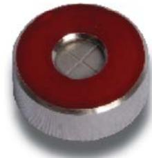
The HTP Igniter is constructed with a stainless steel closure disc that is laser welded into the assembly. This provides a one piece, hermetically sealed enclosure to protect and preserve the explosive primer for extended life and high reliability under harsh conditions. The units are leak tested and labeled with the lot number to meet quality assurance and traceability standards. Two sizes are available to fit standard primer holders.
