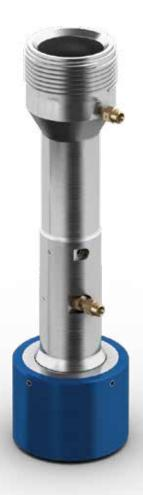
The Hunting Liquid Seal Head is used in conjunction with a conventional Hydraulic Slickline Stuffing Box to create the primary seal on a slickline, while maintaining pressure integrity when running in and out of the well.
