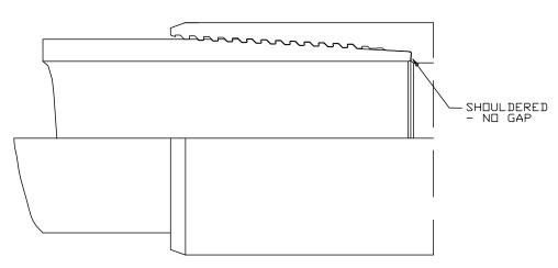
MAKE-UP INSPECTION OF SEAL-LOCK APEX
