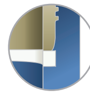
Metal-to-metal seal with optional seal ring for plastic-coated applications
