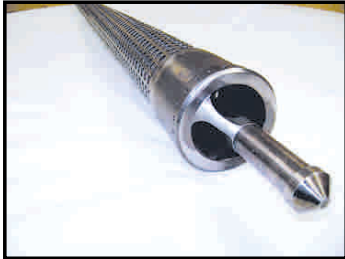
“Premium” Perforated Cone Style Drill Pipe Screen, 3’ Long, Standard Weight 11 Gauge 304 SS, 3/16” Holes - With Extended Collar
