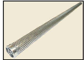
Perforated Cone Style Drill Pipe Screen, 3’ Long, Standard Weight 11 Gauge 304 SS, 3/16” Holes
