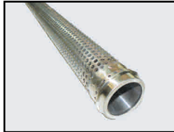
Perforated Cone Style Drill Pipe Screen, 3’ Long, Standard Weight 11 Gauge 304 SS, 3/16” Holes
